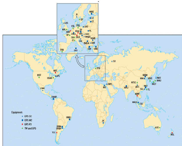
Figure 8. Current configuration of the time links between laboratories and the techniques used for the computation of TAI.
